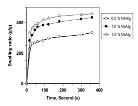
Figure 1. Effects of immersing time on the swelling ratio of NaAlg -g- poly (potassium acrylate) hydrogels at different NaAlg concentrations (0.5% until 1.5%) prepared at irradiation dose 10 kGy.
