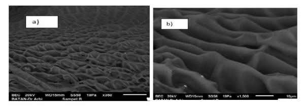
Figure 8. The scanning micrograph of the surface of NaAlg-g- (potassium acrylate) hydrogels prepared by using irradiation were taken with a magnification ; a) 350x and b) 1500x (the scale bar are 50 µm and 10 µm)
